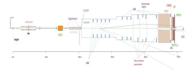
Figure 1: Layout of the NA62 experiment.
