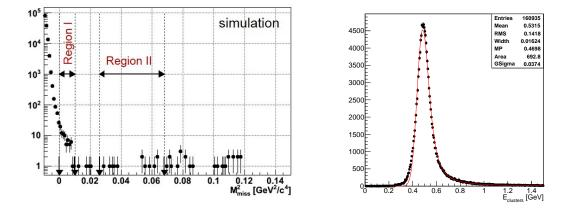
**Figure 4:** Distribution of the reconstructed  $m_{miss}^2$  obtained from simulation for  $K^+ \rightarrow \mu^+ \nu$  (left). The cut on the track momentum is applied. The effect of the pileup on the tails is not included. Energy release of MIP particles in the LKr reconstructed from data taken during the 2012 technical run of NA62 (right). The fit of the energy distribution to a Landau function is superimposed.
