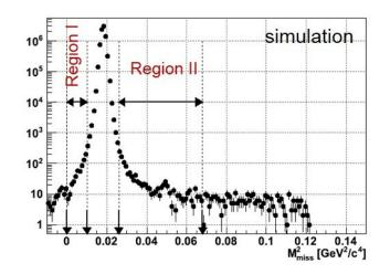
**Figure 3:** Distribution of the reconstructed  $m_{miss}^2$  obtained from simulation for  $K^+ \to \pi^+ \pi^0$ . The events with a  $\pi^+$  decay are rejected by the requirement on pion identification. The effect of the pileup on the tails is not included.
