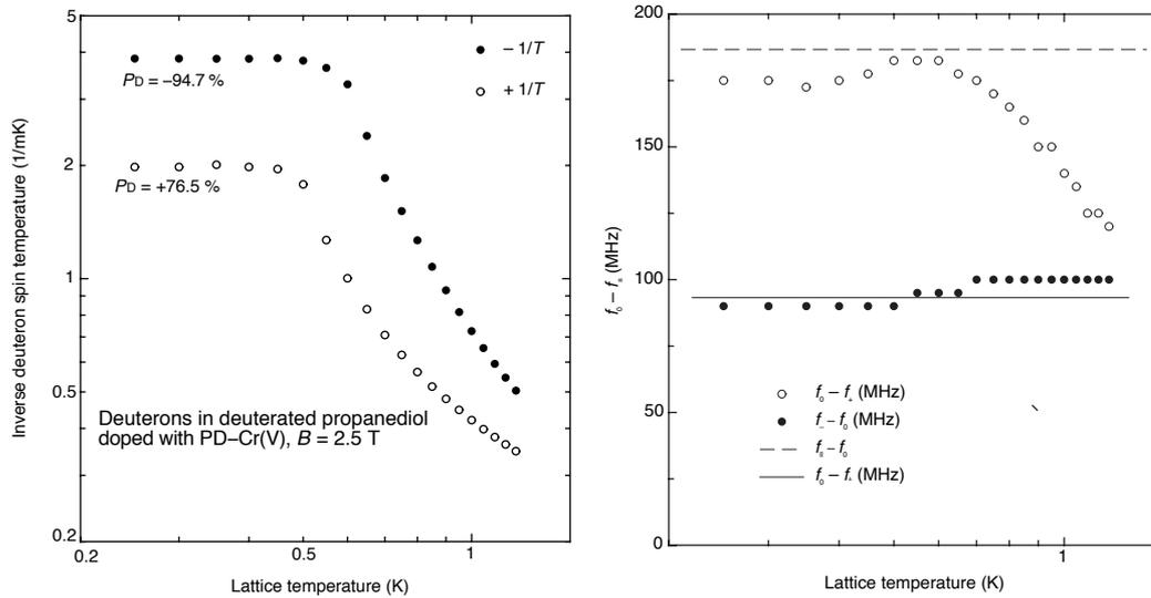
Figure 1: Ultimate DNP in deuterated propanediol doped with PD-Cr(V) [14]. Left – Optimum inverse deuterium spin temperatures as a function of lattice temperature in 2.5 T field; Right – optimum microwave frequencies as a function of lattice temperature. No leakage relaxation is assumed.
