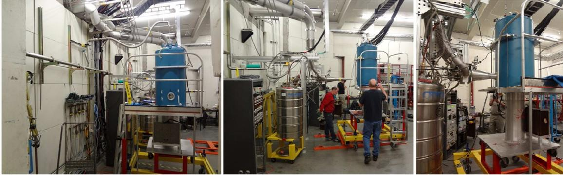
Figure 2. The 2.5T polarizing magnet was filled with LHe (left), rolled the magnet assembly near to the target area (middle), and then aligned the magnet with respect to the target (right).
