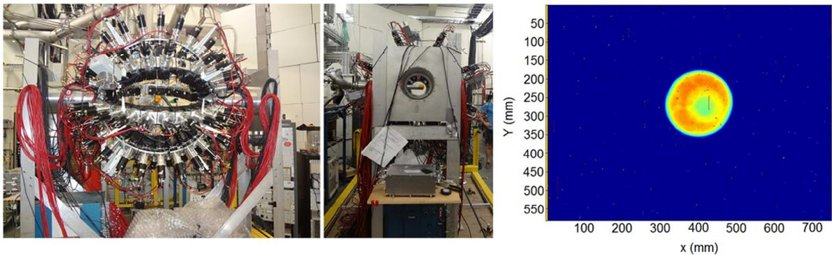
Figure 3. The dilution refrigerator was aligned with the neutron detector array. It was seen from the front (left) and from the side (middle). The target image with a photon beam is in right.
