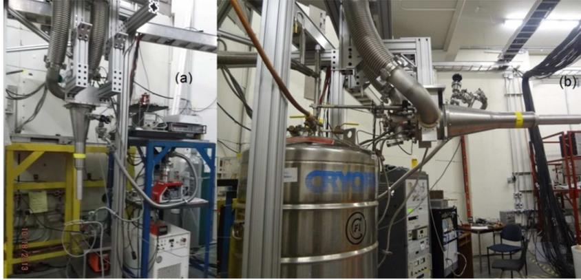
Figure 1. A target stand supports the dilution refrigerator on the beam line both (a) vertically for target changes and (b) horizontally for operation.
