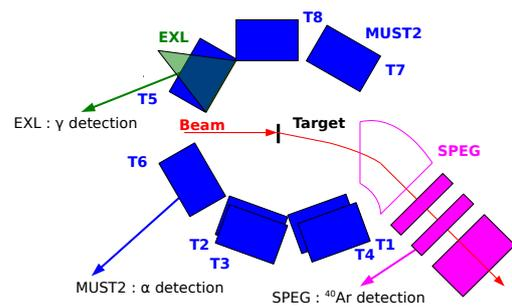
**Figure 2:** Schematic view of the experimental setup.
