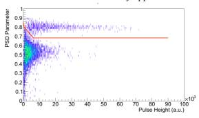
Fig.2 Typical PSD plot from the 4-He detectors showing the discrimination between neutrons (above the red line) and gamma rays (below the red line) from a <sup>252</sup>Cf source.
