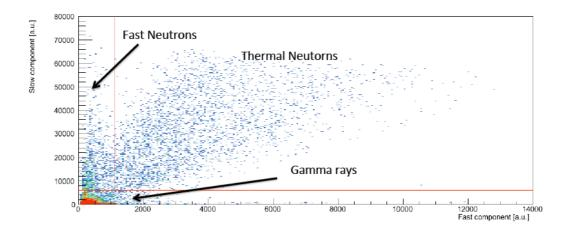
Fig.3 Discrimination of fast and thermal neutrons in the thermal neutron detector.
