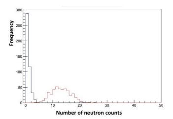
Fig.6 Frequency distribution of neutron counts for 2s sampling windows for the natural background (blue line) and <sup>252</sup>Cf source (red line). For details see the text.
