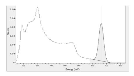
Fig.4 Typical gamma ray spectrum from a <sup>137</sup>Cs source measured with the MODES\_SNM Xe scintillation detector. The energy resolution is about 6% at 662 keV.
