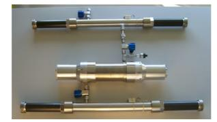
Fig.1 MODES\_SNM detectors: fast neutron (top), gamma ray (middle) and thermal neutron(bottom) .
