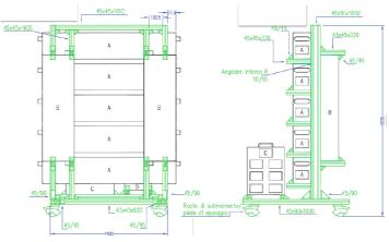
Fig.8 Lay-out of the MODES\_SNM detector array. The vertical boxes contain the gamma ray detectors.
