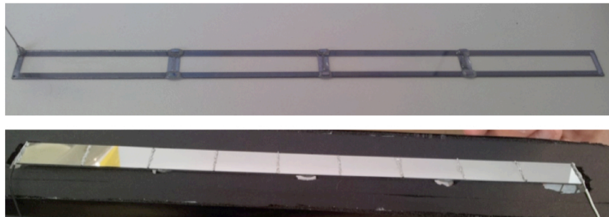
Figure 6 - The first prototype of full stave cooling system with silicon frames with embedded microchannels and distribution lines (top picture) equipped with 9 15 \times 30 \text{ mm} 100 \mu\text{m} thick silicon dummy chips (bottom picture).
