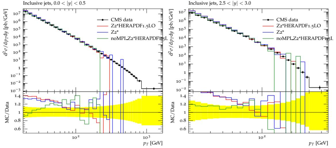
**Figure 3:** Comparison of predictions from PYTHIA using HERAPDFLO1.5 and CTEQ6L for the  $p_T$  spectrum of inclusive jets at central rapidity (left) and forward rapidity (right) to CMS data
