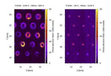
**Figure 10:** Image taken with the Leopard high resolution scanning system. The left image maps the photon sensitivity of a TGEM, whereas on the right, the photons which pass through the holes, and thus measured only by the CCC, are still well detectable.
