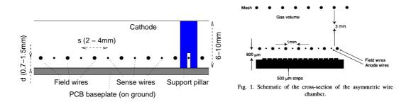
**Figure 1:** Left panel: Outline of the CCC detector. The larger gap acts as charge collection (drift) region, whereas on the side of the lower, thinner gap the baseplate (on ground) may be segmented. Right panel: detector design from [3].
