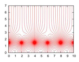
**Figure 5:** Field line distribution in the "Close Cathode" chamber prototype. Electrons are drifting from the upper charge collection zone towards the sense wires (positions 0, 4, 8), whereas the electric field is reduced close to the bottom ground plane due to the concentration of the lines between the field- and sense-wires.
