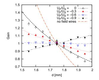
**Figure 3:** Relative gas amplification as a function of lower cathode and wire plane distance *d*, with different  $U_F/U_S$  voltage ratios, at an approximately constant gain at the midpoint. The independence on *d* is clearly demonstrated at  $U_F/U_S \approx -0.6$ .
