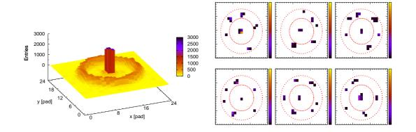
**Figure 9:** Left panel: Cherenkov photons accumulated in a TCPD detector. Right panel: Single events showing identifiable ring patterns
