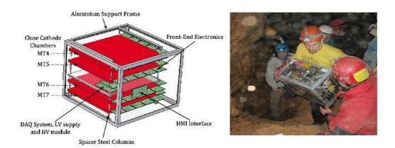
**Figure 8:** Underground detector constructed from CCC tracking layers (left) and deployment to a recently discovered natural cave (right)
