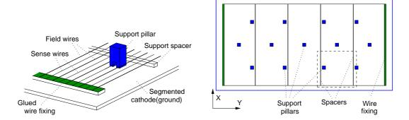
**Figure 7:** Left panel: Mechanical structure inside the CCC chamber. Wire fixations hold the wires in place, while wire supports and pillars should be introduced for large area detectors. Right panel: Schematic top view of the arrangement of the pillars and the spacers on the whole surface of the large prototype chamber.
