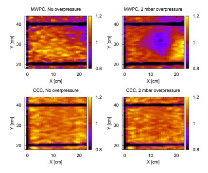
**Figure 4:** Gain measurement (relative, color coded) using cosmic muons over an approximately 20 cm by 20 cm region of the 1 meter chamber (region marked on Fig. 7). The left panels are without, the right panels are with 2 mbar internal overpressure. The top two panels were recorded with the "MWPC" voltage setting, whereas the bottom panels in the "CCC" mode. Note the reduced gain variations for the CCC arrangement.
