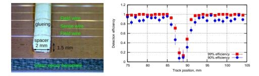
**Figure 6:** Left panel: Intermediate wire fixing spacer for reducing effective wire length. Right panel: Detection efficiency as a function of position in the chamber prototype, in the vincinity of the 2 mm wide intermediate spacer.
