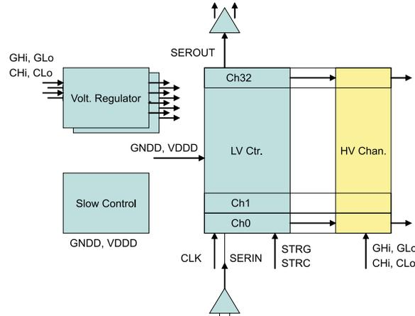
**Figure 3:** Block diagram of the SWITCHERB chip.
