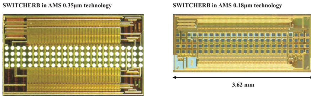
**Figure 4:** Photomicrograph two SWITCHERB versions. Left picture shows the chip implemented in 0.35  $\mu\text{m}$  AMS technology, right picture shows the chip in 0.18  $\mu\text{m}$  technology.
