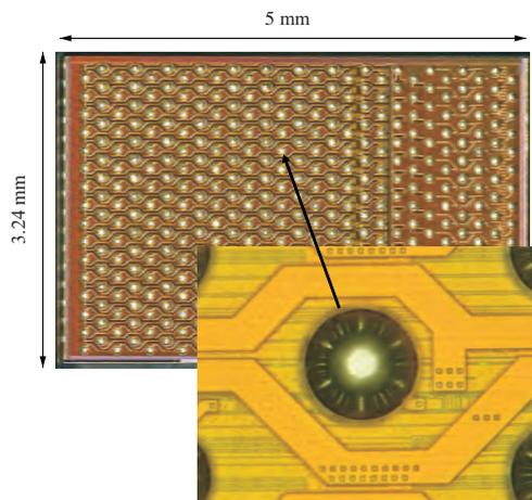
**Figure 2:** Photomicrograph of the DCDB chip.
