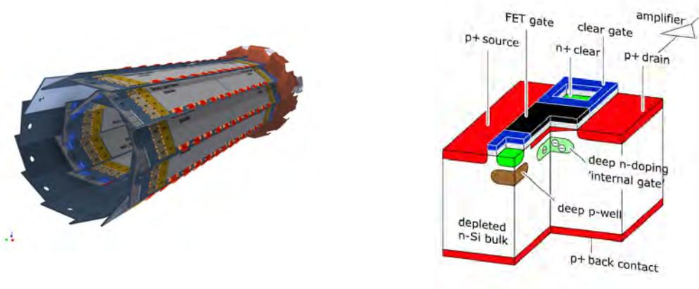
**Figure 1:** (Left) Geometry of the Belle II PXD which consists of two layers of DEPFET sensor modules. (Right) Cross-section of a DEPFET sensor consisting of a p-channel FET on a sidewall depleted silicon bulk.
