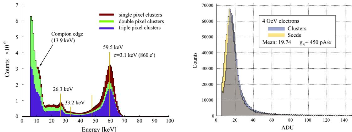
**Figure 7:** (Left) Spectrum of  $^{241}\text{Am}$  obtained with the trigger-less mode. (Right) Histogram of the signals from 4 GeV electrons.
