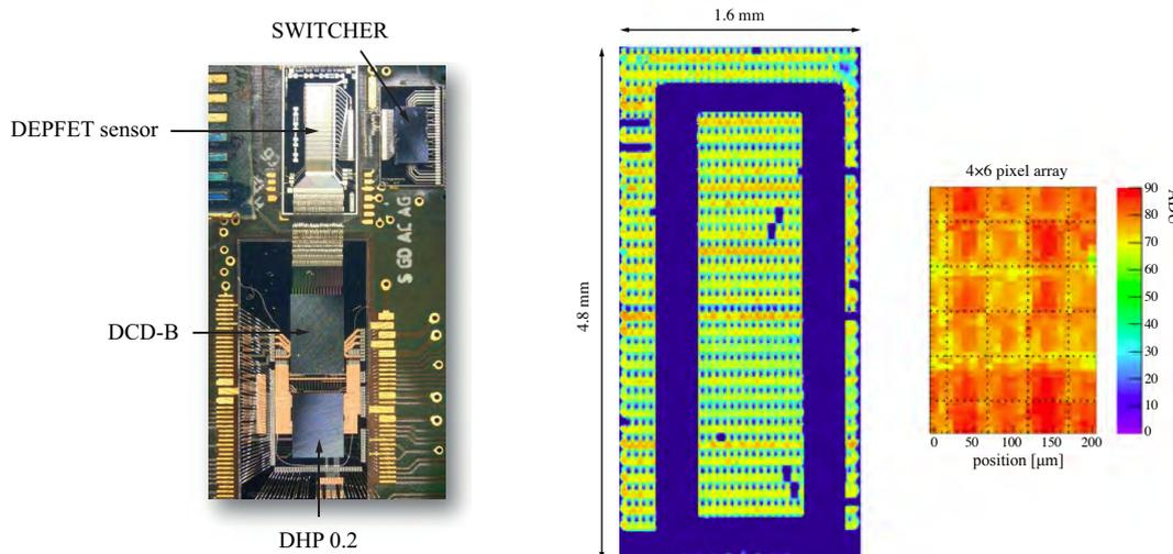
**Figure 6:** (Left) A picture of the full-scale module prototype, including a small DEPFET matrix, one SWITCHER, one DCDB, and one DHP0.2. (Right) The matrix image of the laser scan from the back-side. The metallization area can be seen as a blue rectangle. Right picture shows a precise homogeneity scan result of the  $4 \times 6$  pixel area with a step of  $10 \mu\text{m}$ .
