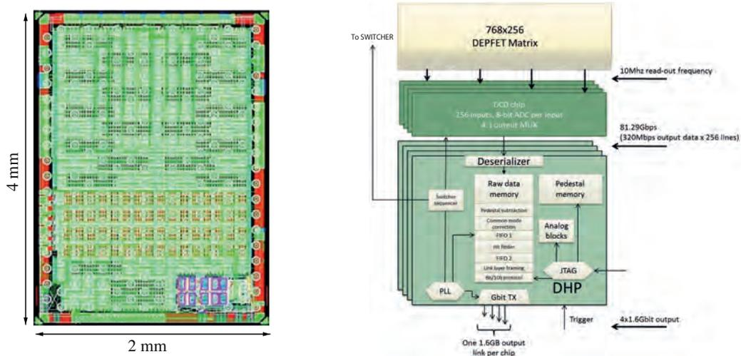
**Figure 5:** (Left) A layout of the newly developed DHP chip with TSMC 65 nm CMOS. (Right) Block diagram of the DHP chip.
