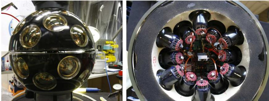
**Figure 2:** The KM3NeT Digital Optical Module (DOM).
