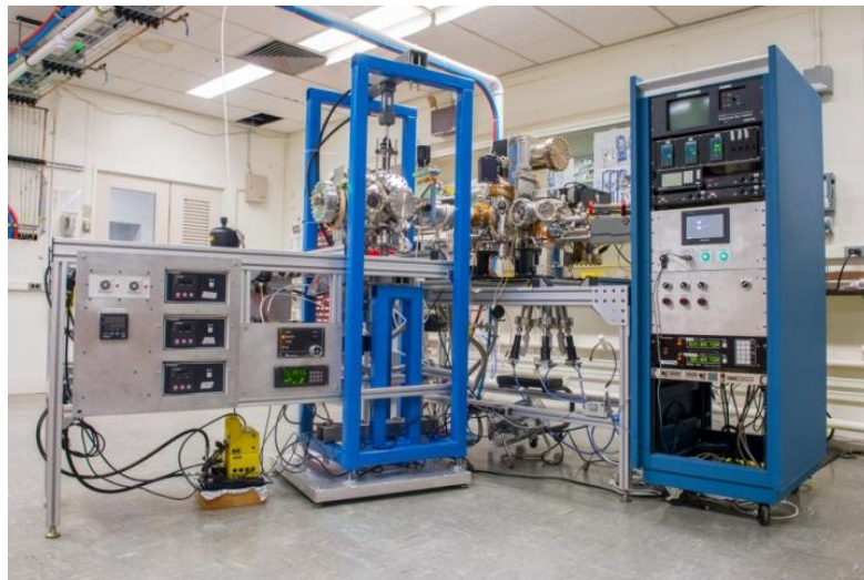
Figure 2. Picture of the constructed 6 cm x 6 cm small single tile photodetector production facility at Argonne National Laboratory.
