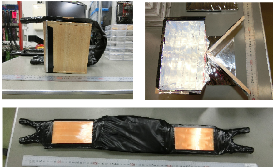
Figure 1: Prototype of multipurpose aerogel Cherenkov counter. The fiber light guide is set at a space of not irradiated directly from particles and the effective area is 120 \times 100 \text{ mm}^2 as can be seen from the front view (top left). Cherenkov light emitted from the aerogel is reflected by a V-shaped reflector and collected into the fiber light guide as can be seen from the side view (top right). The fiber light guide has two surfaces of the effective area of 60 \times 100 \text{ mm}^2 (bottom).
