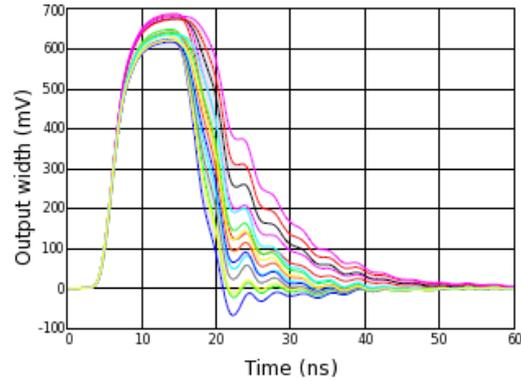
Figure 4: Amplifier response to large signals (150 fC) showing short recovery time.
