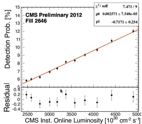
Figure 2: Sensor hit probability with instantaneous luminosity.
