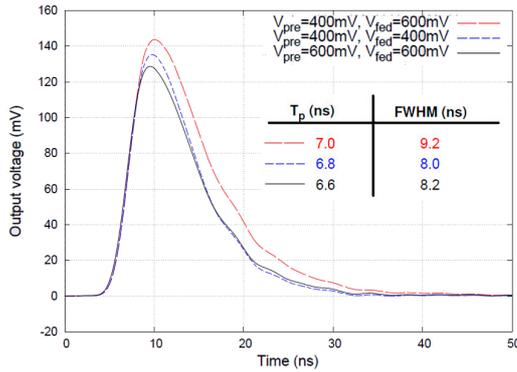
Figure 3: Amplifier response to MIP signals showing fast rise time for various bias settings.
