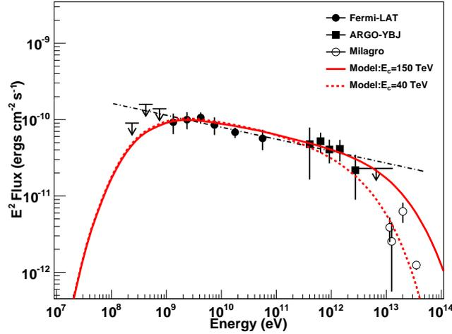
**Figure 5:** Spectrum of the Cygnus Cocoon as measured by different detectors. The arrows below 1 GeV indicate the upper limits set by Fermi/LAT, the Milagro data refer to MGRO J2031+41, at 12 TeV corrected for the extrapolation of TeV J2032+4130 [17]. The dot-dashed line shows the power law best fit to the combined Fermi/LAT and ARGO-YBJ data. The solid and dotted curves are predicted by a purely hadronic model with proton cutoff energy at 150 TeV and 40 TeV, respectively.
