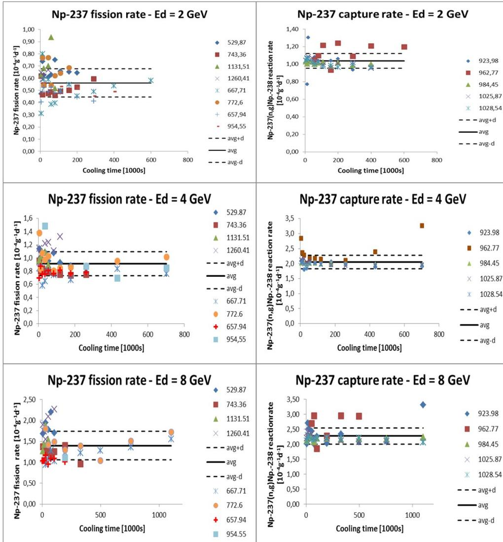
Figure 5. Np-237 fission and capture rate based on identified gamma lines for beam deuteron energies 2, 4 and 8 GeV. Solid and dashed lines show  $\pm \sigma$  (standard deviation of population) range.
