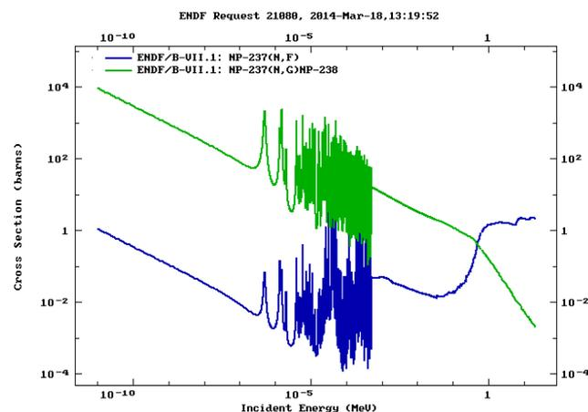
Figure 1. Np-237 neutron caused fission (dark blue) and capture (green) cross section dependence on energy [2].
