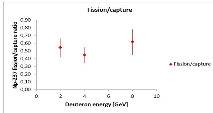
Figure 7. Np-237 fission to capture ratio dependence on beam deuteron energy
