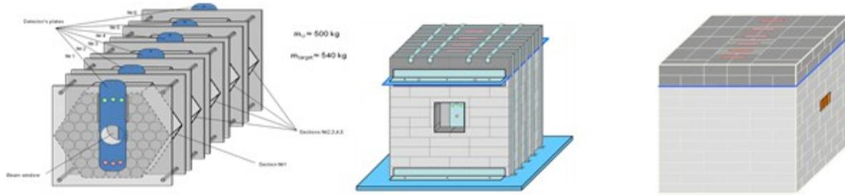
Figure 2. QUINTA setup view - internal core, front view and rear view.
