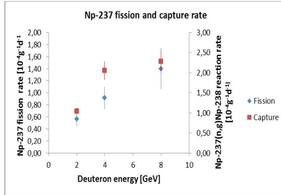
Figure 6. Np-237 average fission and capture rate per gram and per 1 deuteron dependence on energy
