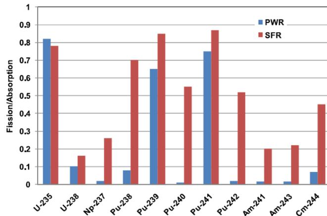
Figure 8. Actinides fission to absorption ratio for PWR and SFR [1]
