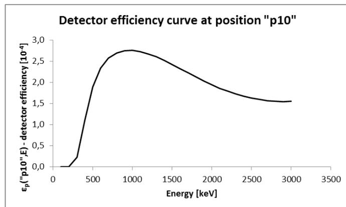
Figure 4. HPGe detector efficiency dependence on energy
