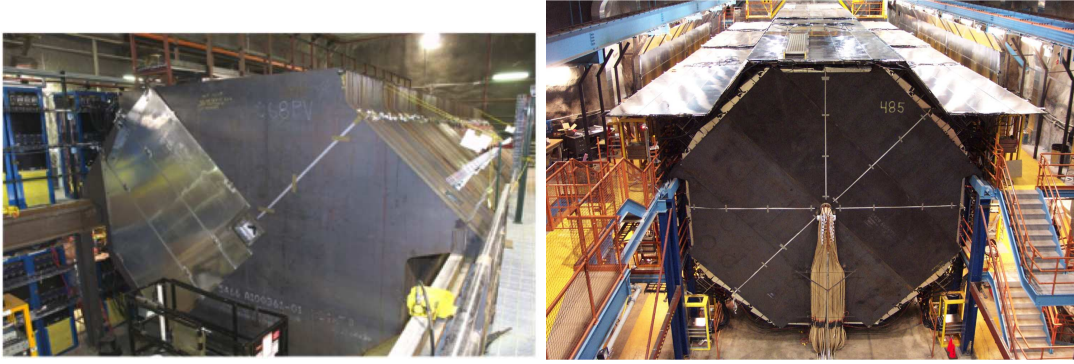
Figure 1: Pictures of the two MINOS+ Detectors. The Near Detector is smaller, at about 1 kT mass and 15 m length. The Far Detector is very large at 5.4 kTon mass and 30 m length, and has a veto shield above it to identify cosmic ray muons.
