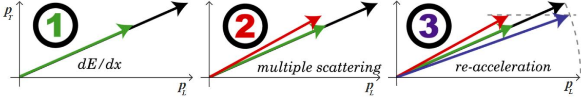
Figure 1: An illustration of ionization cooling.
