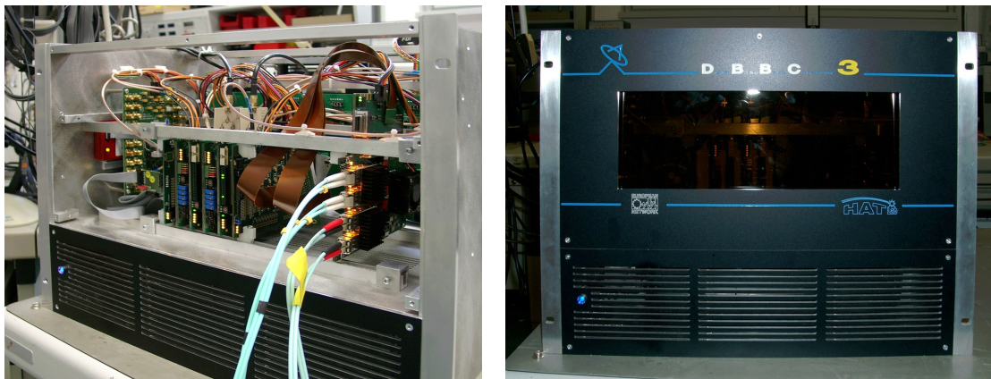
Fig. 5: Left: Internal view of the DBBC3. In the centre the stack with the two ADB3-L and CORE3-L can be seen. Right: Front view of the DBBC3.
