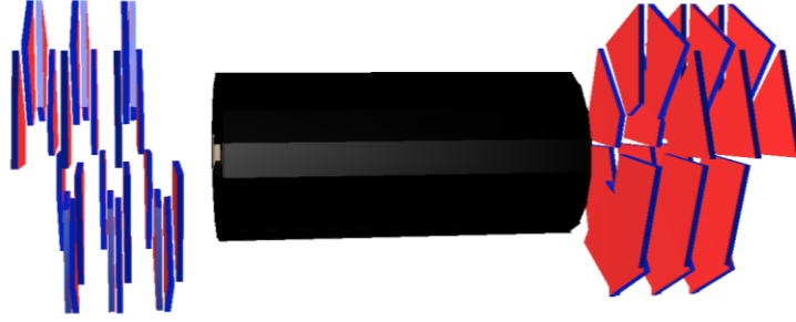
Figure 6: Schematic representation of the vertex detector at CLIC, as presently implemented in the simulations. The central vertex barrel (in black) is 26 cm long and consists of three double-layers. To allow for efficient air-flow cooling, the end-caps are built as spirals, also forming three double-layers.
