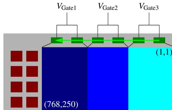
Figure 2: The DEPFET sensor can be supplied with three different gate voltages  $V_{\text{Gate}1-3}$ . That way we can account for irradiation-induced shifts of the operation point. The green boxes symbolize the “Switcher” chips, which apply the gate and clear voltages consecutively to the pixel rows, and the red boxes symbolize the “Drain Current Digitizer (DCD)” and “Data Handling Processor (DHP)” chips, which read the drain currents and perform processing.
