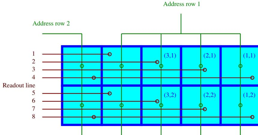
Figure 3: The “four-fold readout” scheme addresses four pixel rows at the same time. This scheme reduces the total frame time by a factor four, and increases the necessary number of readout channels by a factor four.
