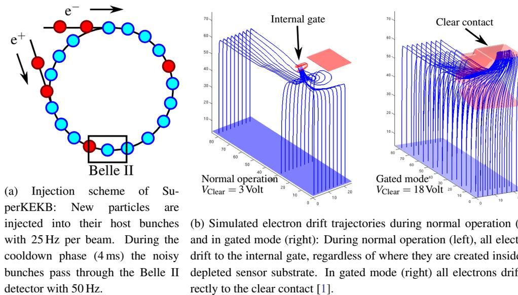
Figure 4: The injection scheme of SuperKEKB (4a) makes it necessary to shield the PXD against noisy bunches. This is achieved with the “gated mode” operation (4b).
