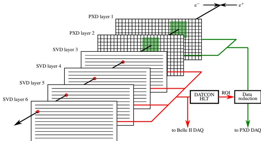
Figure 5: Background suppression for the PXD: The Silicon Vertex Detector (SVD) tracks particle trajectories with high timing accuracy (red circles), yielding a prediction of where the particle should have left a hit on the PXD sensors. Around these predicted hit positions we define “Regions of interest” (ROIs, green squares). Only hits inside these ROIs are read out.
