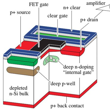
Figure 1: Principle of a DEPFET pixel: A field effect transistor (p+ source, FET gate, p+ drain) sits on top of a depleted silicon substrate. Particle-induced electrons are collected in the internal gate and modulate the drain current. The stored electrons are removed via the n+ clear contact.
