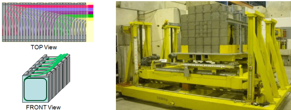
Figure 1: (left) Module design of the forward calorimeter. (right) An image of the NA61/SHINE PSD.
