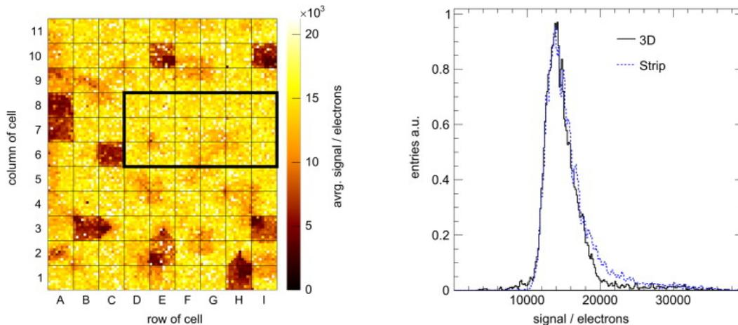
**Figure 4:** Selected region of the 3D detector (left) and collected charge in said region compared to the charge collected in the 2D planar strip detector (right).
