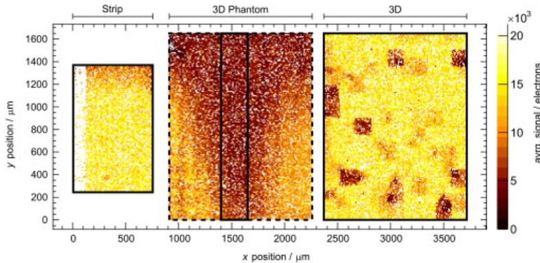
**Figure 2:** Measured charge on the 2D strip (left), 3D phantom (center), and 3D (right) detector geometries.
