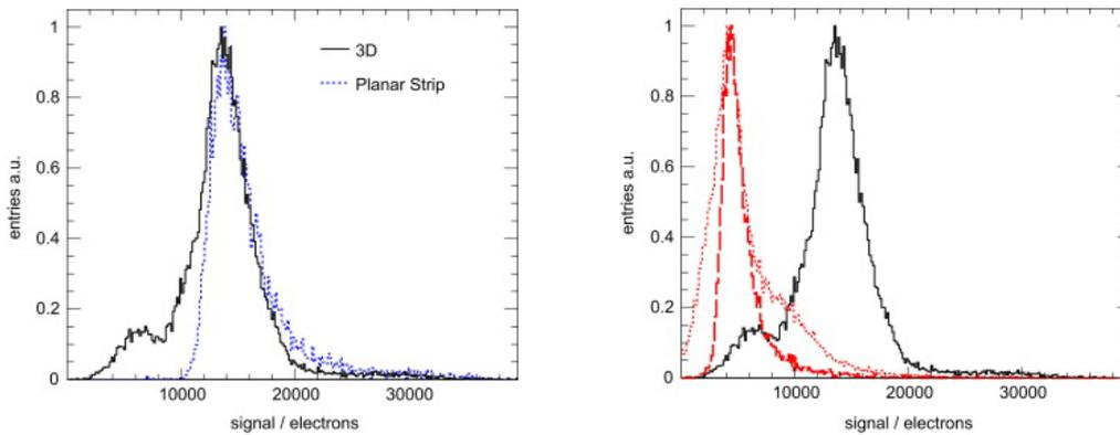
**Figure 3:** Comparison of measured charges in the 3D detector and 2D strip detector (left) and of the 3D detector and the 3D phantom detector (right). The 3D detector charge is shown shown as a black solid line and all distributions are scaled to the same peak height. The dashed line in the right plot indicates only the central region of the 3D phantom detector, while the broad solid line represents all charges in the 3D phantom detector.
