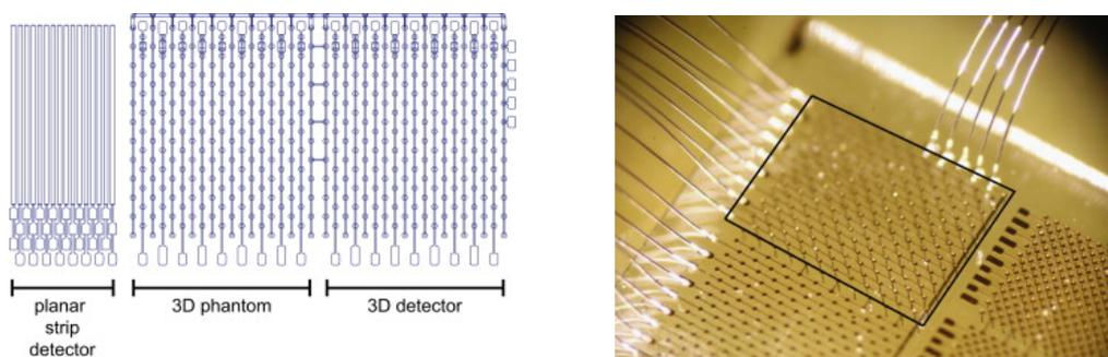
**Figure 1:** Schematic drawing of the prototype 3D diamond sensor and metallization (left). Photograph of the diamond sensor after metallization and wire-bonding (right).
