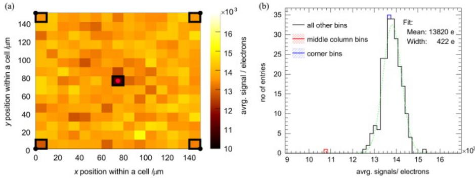
**Figure 5:** Overlay of the signal collection in sub-cells as a 2D distribution (right) and a 1D distribution (left).
