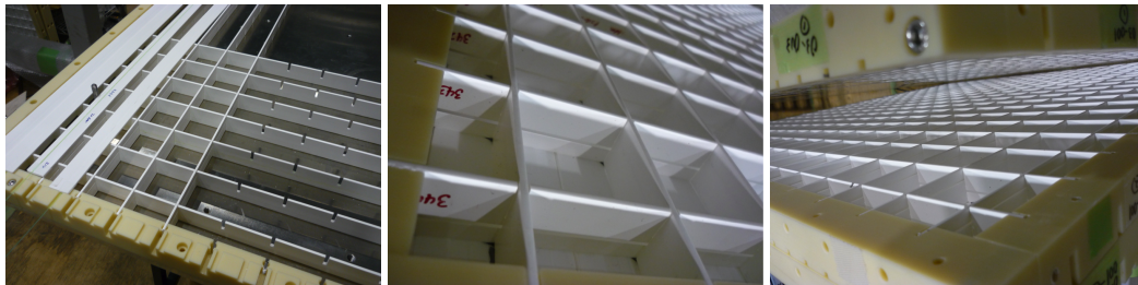
Figure 2: WAGASCI plastic scintillator 3D grid structure. Dimensions of each cell are 5 \times 5 \times 2.5 \text{ cm}^3 . The cells are filled with either H 2 O or CH to form the neutrino interaction target of the experiment.
