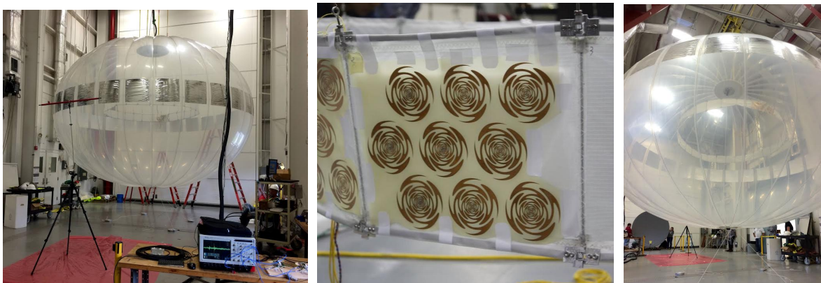
Figure 7: Left: Fully deployed 20 ft diameter balloon, and DAQ system in foreground. Center: detail of sinuous patch antenna array. Right: view of fully deployed internal feed array, from below the balloon.
