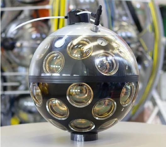
**Figure 1:** The KM3NeT Digital Optical Module.
