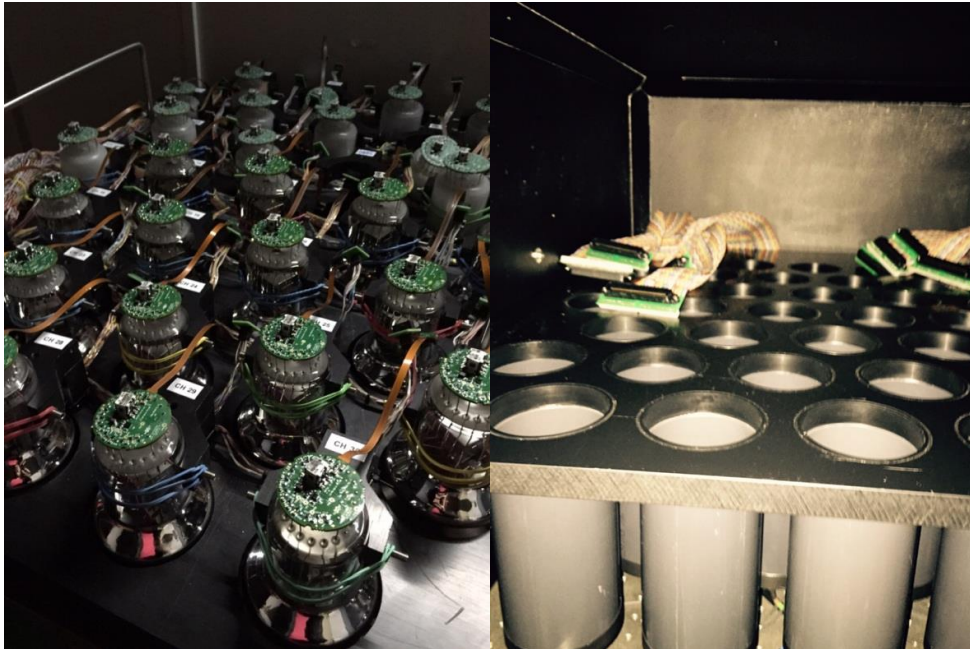
Figure 2: PMTs in the tray before the test (left). The DarkBox inner structure (right)
