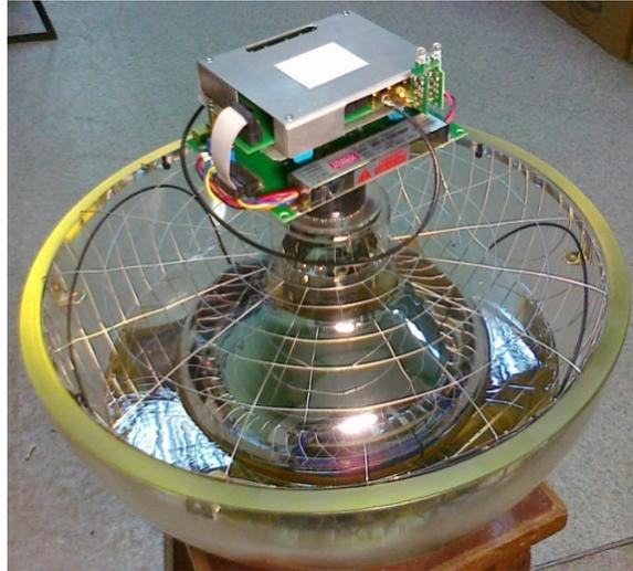
**Figure 4:** Picture of the Baikal-GVD Optical Module. Two LEDs are seen at the top of the OM electronics.
