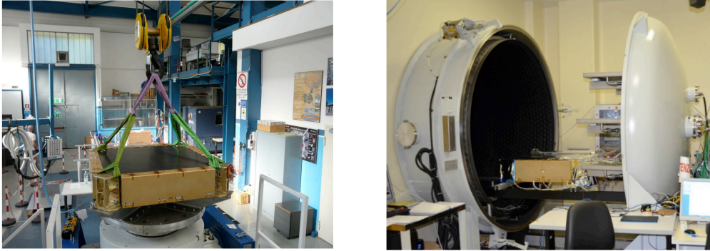
Figure 9: The STK EQM being installed for vibration (left) and thermal vacuum tests in SERMS, Terni, Italy.
