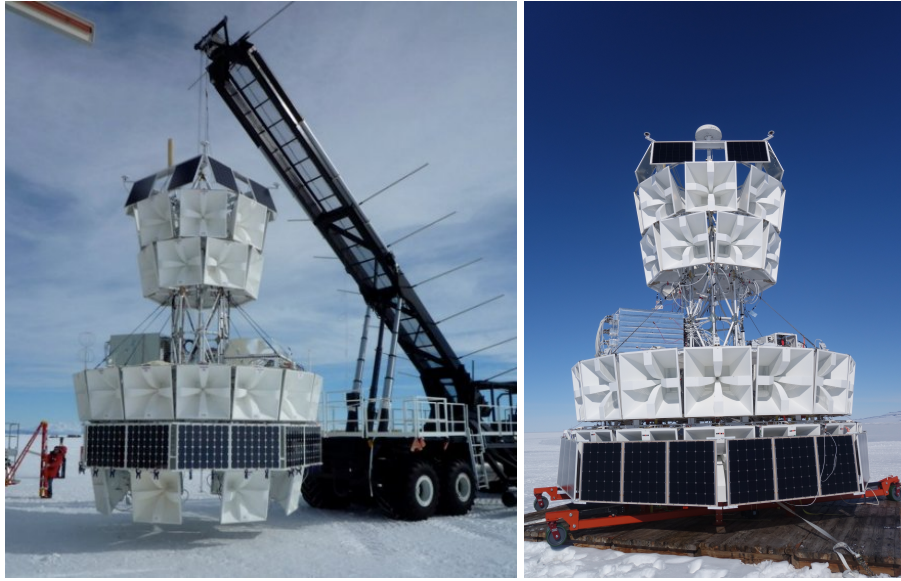
Figure 2: The ANITA2 (left) and ANITA3 (right) instruments before launch. ANITA 2 is seen hanging from launch vehicle at the Long Duration Balloon Facility outside McMurdo Station Antarctica, 2008. The eight nadir ring antennas, stowed for launch, are deployed in this photo (Photo courtesy of Ryan Nichol) The ANITA3 instrument is seen sitting on a testing "dance floor", also outside McMurdo Station, Antarctica, in 2015. Note that the nadir ring of 16 antennas is obscured by the stowed solar panel ring.(Photo by author)
