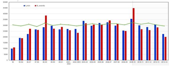
**Figure 1:** Small Cherenkov array. Statistics of showers with energy more than  $2 \cdot 10^{15}$  eV. Blue bars - time of observation in minutes. Red bars - number of registered air shower events. Green line - average spectral transparency of the atmosphere for wavelength  $\lambda = 430$  nm
