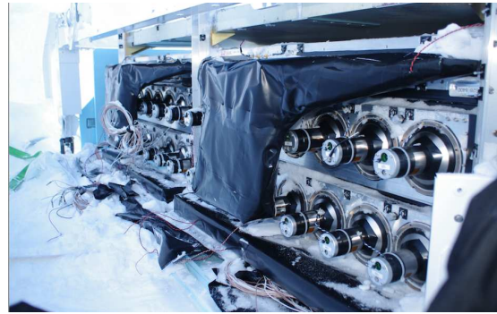
Figure 6: Photo 2 of the recovery site. The HV cables and signal cables were carefully removed from the PMTs.
