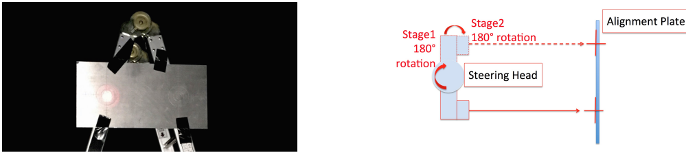
Figure 7: Custom alignment plate (left) used to check alignment of steering head. Two targets are spaced apart to match horizontal displacement of the beam when the 2 stages are rotated by 180^\circ (right).
