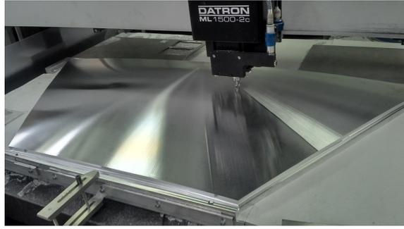
**Figure 4:** Mold manufacturing for central part of the METS mirror.
