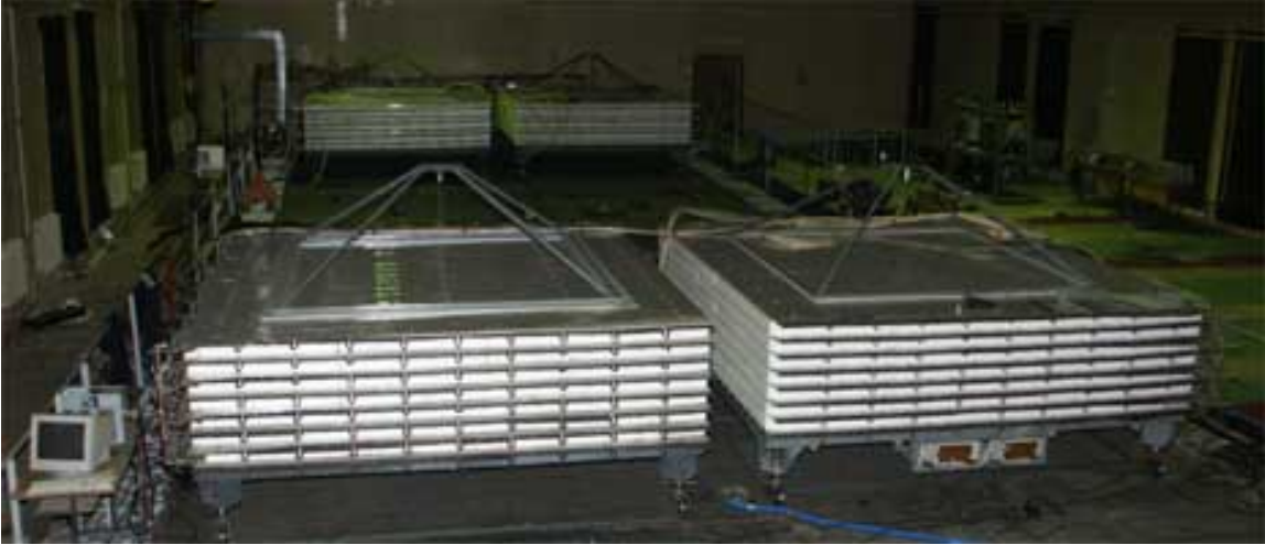
Figure 2: The muon hodoscope URAGAN on top of the NEVOD detector. The four Super Modules are easily distinguishable. Only three of them are taking data regularly. The fourth one is used for testing and calibrating other detectors.
