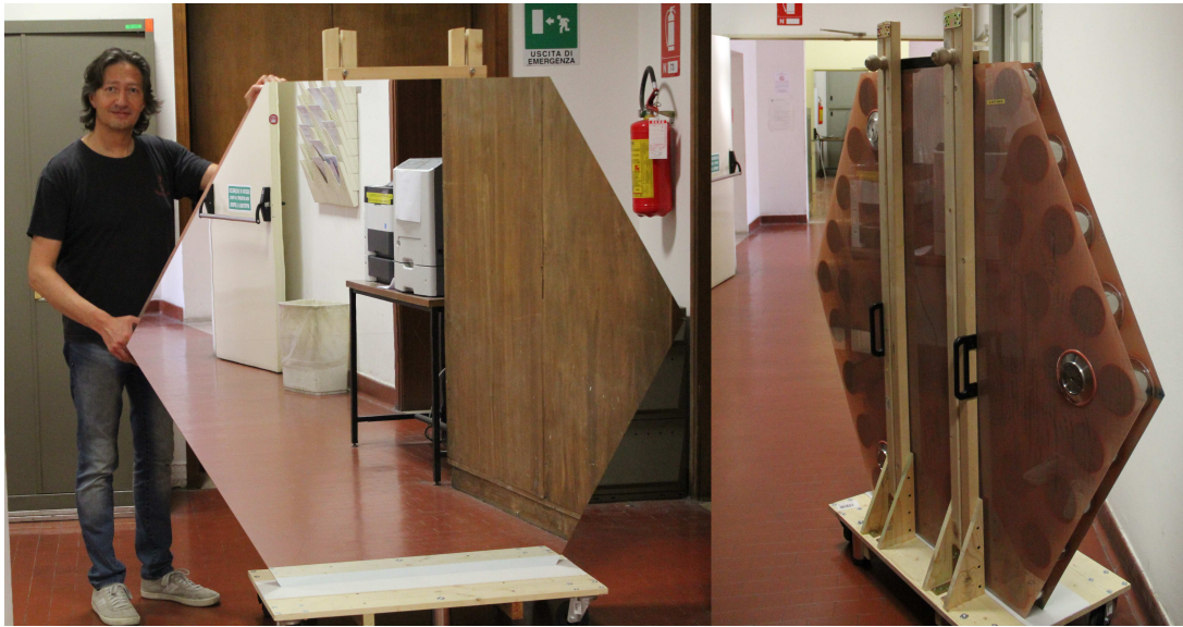
Figure 3: Front (left) and rear (right) of one of the first 1.5 FTF diameter mirror prototypes proposed to be used for the LST.
