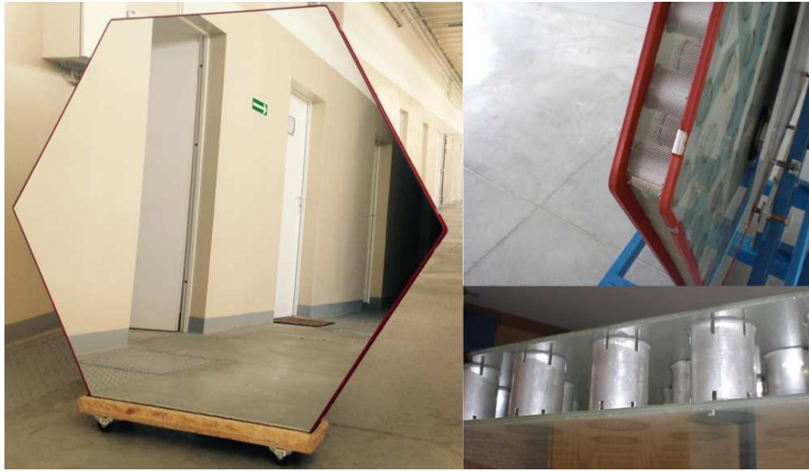
Figure 2: The front of an open structure mirror with reflective layer (left) and the sidewalls with the protective silicon rubber and stainless steel mesh (top right). Visible are the aluminum spacers with slots cut at both ends of the tubes (bottom right).
