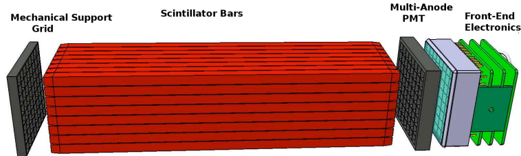
Figure 1: Schematic representation of a single module of POLAR. The scintillator bars are shown in red, together with the MAPMT, the front-end electronics and the mechanical support structure.
