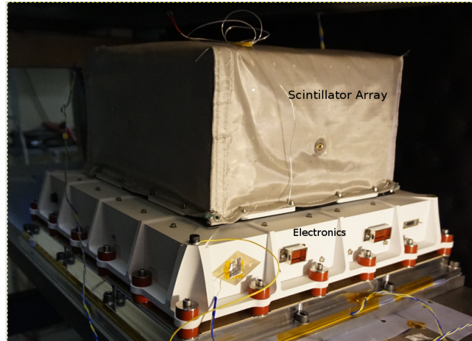
Figure 2: The POLAR flight model during thermal vacuum tests. The electronics is contained in the white painted aluminium structure while the scintillator array is placed in a carbon structure covered with a multi-layer insulator.
