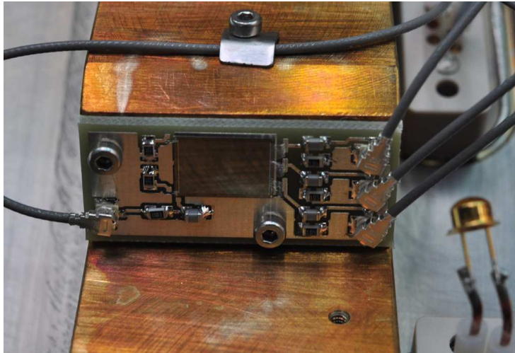
Figure 5: A 5\ \mu\text{m} detector mounted on a printed circuit board as installed on the KF1 vacuum flange prior to installation on the machine. Hirose U-FL-series ultra-miniature connectors are used for bias (left) and AC-coupled signal connections (right). The detector is read-out as three banks of 20 strips. An IR LED for artificial excitation of the detectors is seen at lower left.
