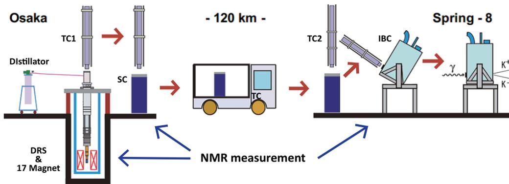
**Figure 1:** Transportation diagram for Polarized HD target from production to installing IBC
