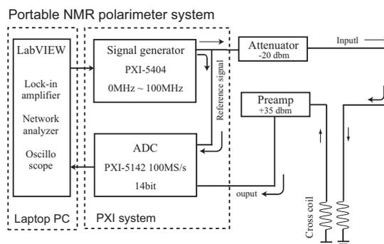
Figure 4: NMR circuit for using 17 tesla NMR monitor
