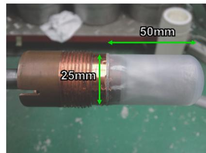
**Figure 2:** The HD target cell without coil for the LEPS experiments. The geometry of the cell is 2.5 cm in diameter and 5 cm in length. The coil frame is covered this target when NMR measurement is performed.
