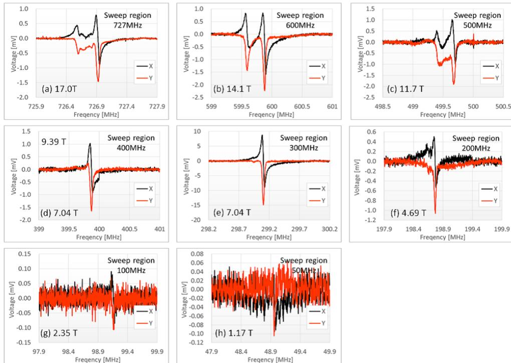
**Figure 5:** Measured NMR signals by frequency sweep from 50 MHz (1.17 Tesla) to 727 MHz (17.0 Tesla). Red curves are absorption signals, and black curves are dispersion signals.
