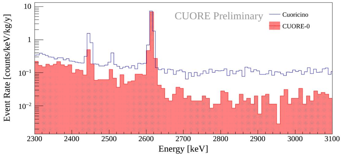
Figure 3: Zoom of the spectra shown in Figure 2 in the energy region across the  $^{208}\text{Tl}$  peak.
