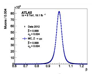
**Figure 1:** Combined  $\beta$  measurement (right) for selected  $Z \rightarrow \mu\mu$  events in data (points) and MC simulation (line) [1].
