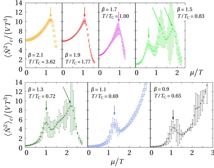
**Figure 4:** The second cumulant of the quark number  $\langle \hat{N}^2 \rangle_c / (VT^3)$  as a function of the quark chemical potential. The lower panels plot results for  $T/T_c = 0.65, 0.69$  and  $0.72$  below  $T_c$ . The upper panel is results for  $T_c = 0.83 - 3.62$ .
