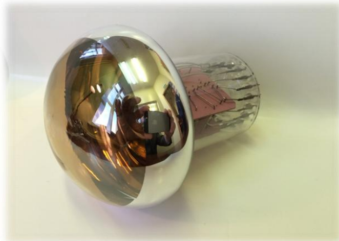
Fig. 2. 3-inch PMT with mushroom shape glass envelope developed for low energy neutrino experiments.
