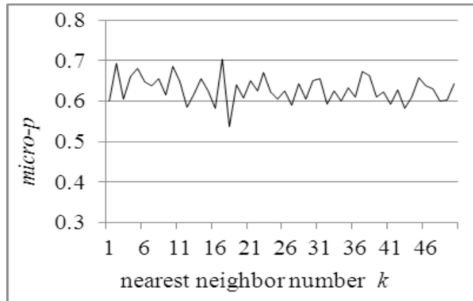
Figure 2: Change of micro-p with Nearest Neighbor Number k in Face Four Dataset
