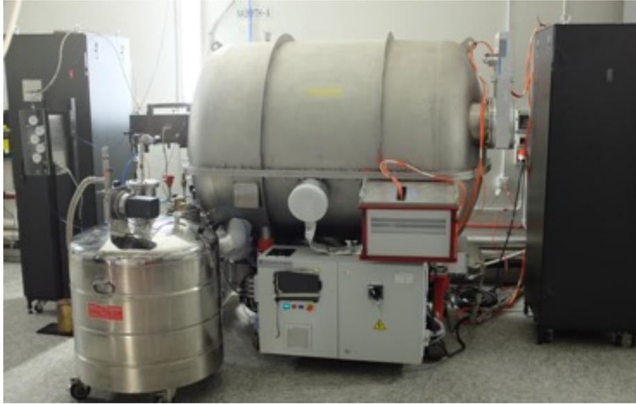
**Figure 2:** GIANO vacuum vessel, fiber agitator, LN2 tank and the electronics in the Nasmyth – A of TNG
