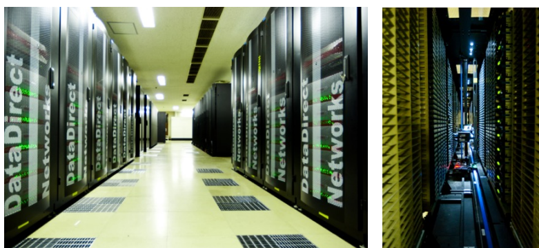
(a) DDN SFA10K: 7 PB of disk storage of which 3 PB is in use for the HSM disk cache. The remaining 4 PB is used directly by the users and experimental groups. (b) IBM TS3500: 16 PB of maximum capacity in the tape library.
