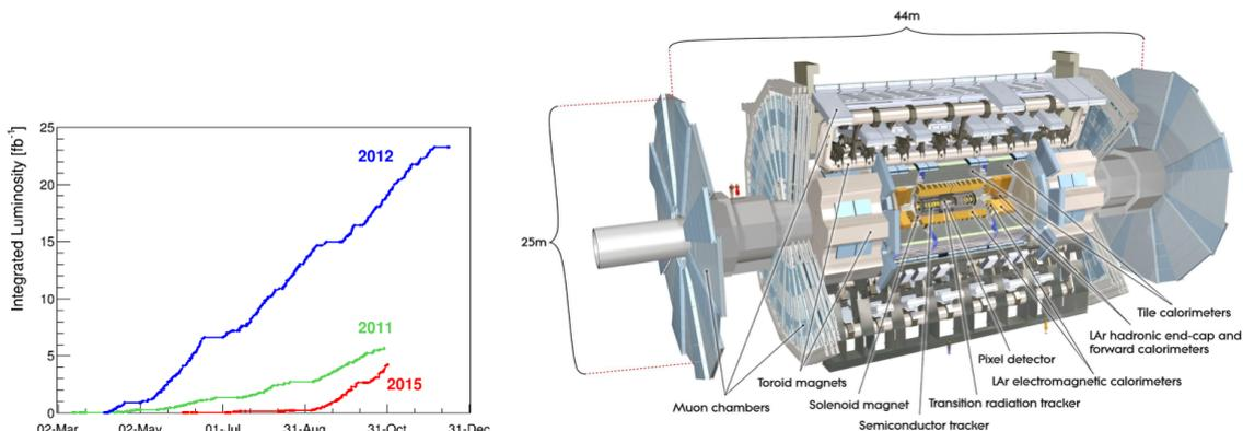
**Figure 1:** History of the integrated luminosity [2] (left) and structure of the ATLAS detector [4] operated at the Large Hadron Collider (right).
