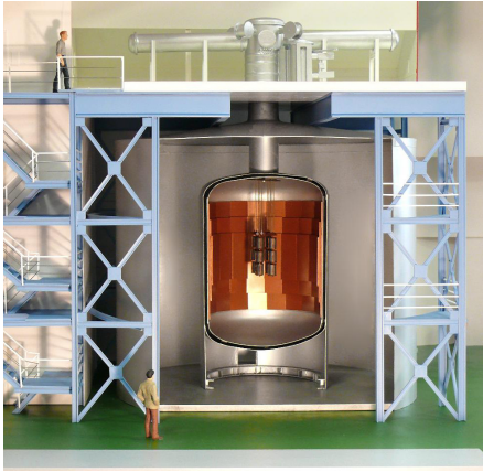
Figure 1: Model of the GERDA design. Visible are the water tank, the LAr cryostat with the ultra-clean copper shield on the wall and the lock system on the top.
