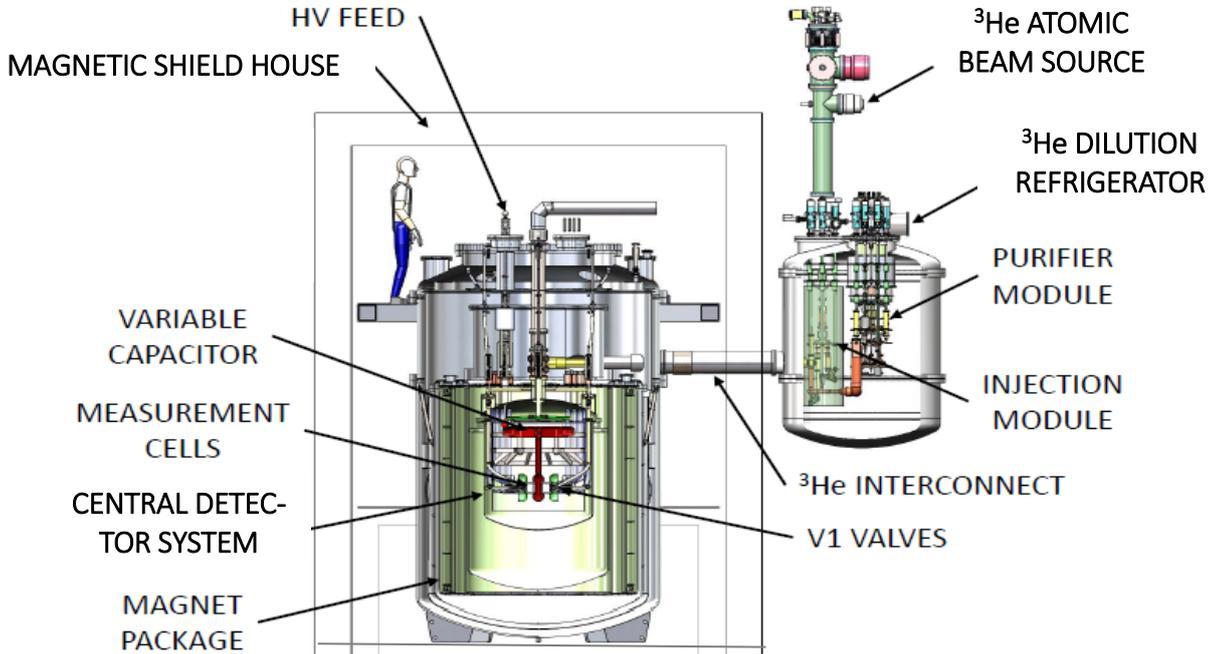
**Figure 2:** Schematic of the nEDM apparatus for measuring the neutron EDM at the Spallation Neutron Source at Oak Ridge National Laboratory.
