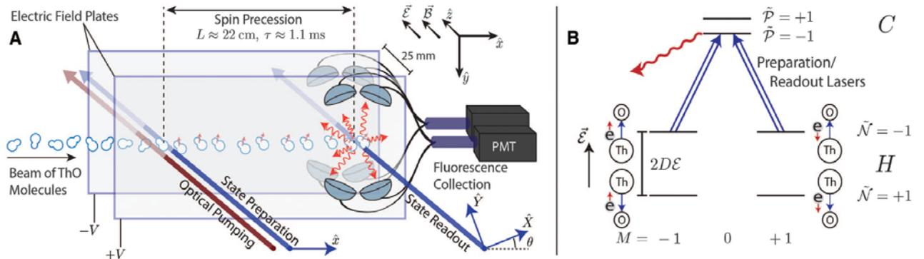
**Figure 1:** **A.** Schematic of the ACME apparatus for measuring the electron EDM. The beam of ThO is prepared and read out with lasers to measure the electric-field-dependent frequency shift that is characteristic of an EDM. **B.** Summary of state preparation of the ThO. The level diagram on the left shows the two states that can be selected where the effective electric field is flipped while the applied electric field is held fixed. Figure from ref [6].
