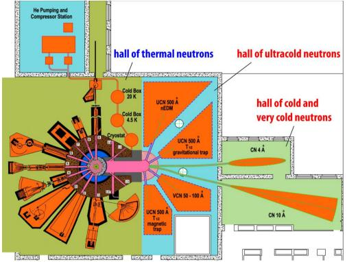
**Figure 3**. Experimental halls of the reactor WWR-M. The location scheme of the source of cold and ultracold neutrons, complex of experimental installations in the main reactor hall and complex of experimental installations in neutron guide halls.
