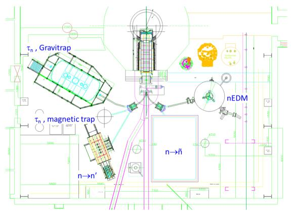
Figure 5. Scheme of experimental apparatus location in the hall of ultracold neutrons of the WWR-M reactor.
